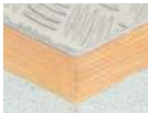
Bonding of floor elements
