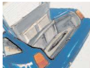
Seam sealing application with Körapop 216
