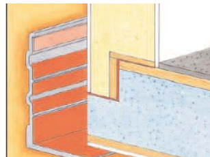
Use of Köratape as an assembly aid
