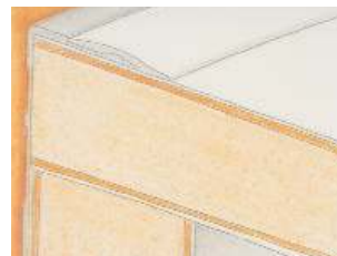
Sealing of a roof element with Körapur 128 / 2-part
