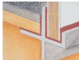
Sealing application with Körapur 125
