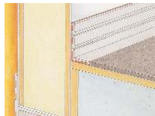
Inside sealing with Körapur 115
