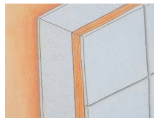
Bonding of a 4-layer sandwich element
