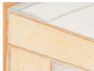
Bonding of a roof-element with Körapur 140
