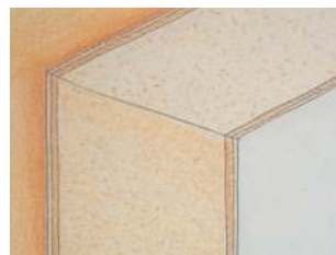
Bonding of 5-layer-sandwich-element
