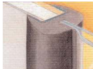
Sealing against water with Ködiplast CT
