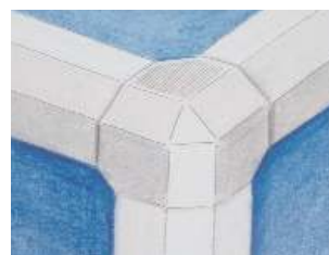
Bonding of edge profiles with Körapur 140 / 2-part
