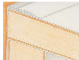
Sealing of a roof element with Körapur 128 / 2-part
