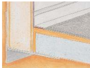
Bonding of a skirting board with Körapur 840
